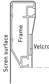
11. When the fabric is attached on top, attach the fabric on the sides. Then rotate the frame and attach the remaining surface at the top.
