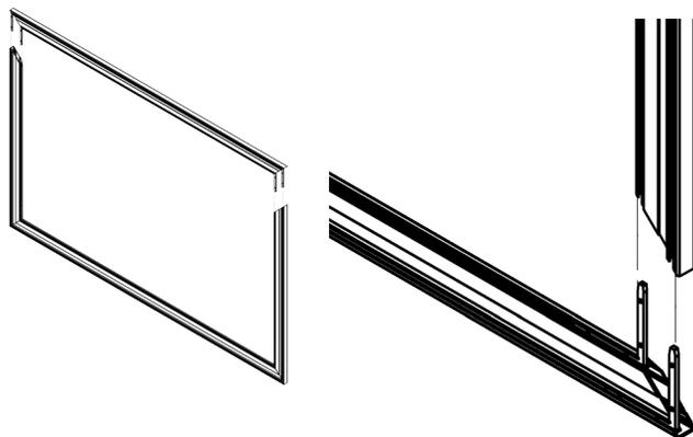
1. Unwrap the frame pieces. Before assembling the frame pieces, add 2 nuts (A) to either end of the top frame section and the top of the side frame for the mounting bracket and add 2 nuts to the bottom frame.
