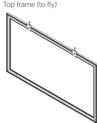
5. Secure the mounting bracket (C) with provided screws to the previously inserted nuts.
