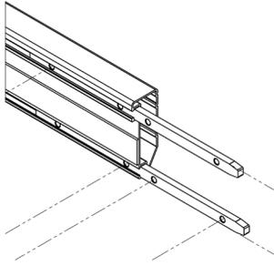
8.2 Screens wider than 400 cm require a spreader bar. Connect the top and bottom frame with the spreader bar and connect this by using the two supplied screws (D).
